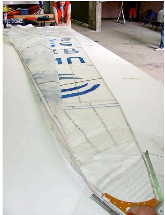
Mark the leech points at leech (see pic below). Check the widths. Check concavities on the leech and sail reinforcements.
