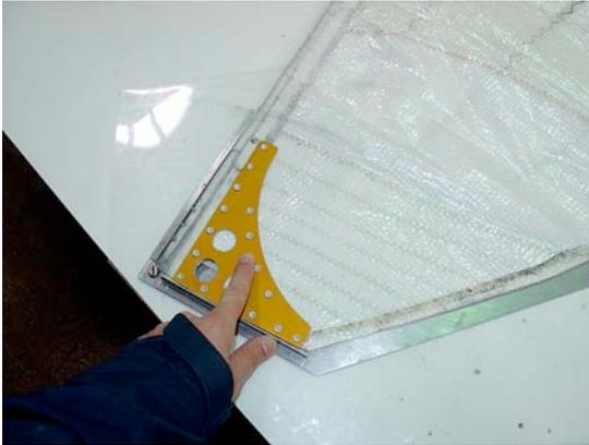
Lay the sail on the table with its head on the gauge (see pic left). The gauge helps to check the width of the headboard, depth of the headboard and primary reinforcement, location of the Aft Head Point and the distance from the 425 mm Upper Leech Point to the luff.
